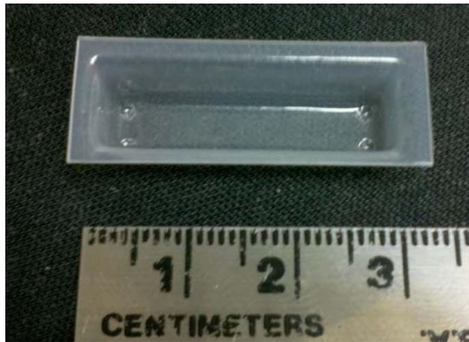
*Figure 2. Polypropylene collimated beam test cup*
