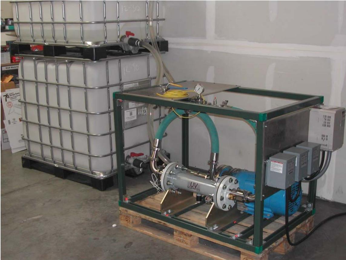
*Figure 5. NeoTech Aqua 170 GPM Flowing Disinfection Test Skid.*
